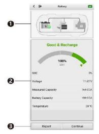
Figure 4-6 Sample Battery Test Result Screen
