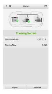
Figure 4-7 Sample Starter Test Results Screen
